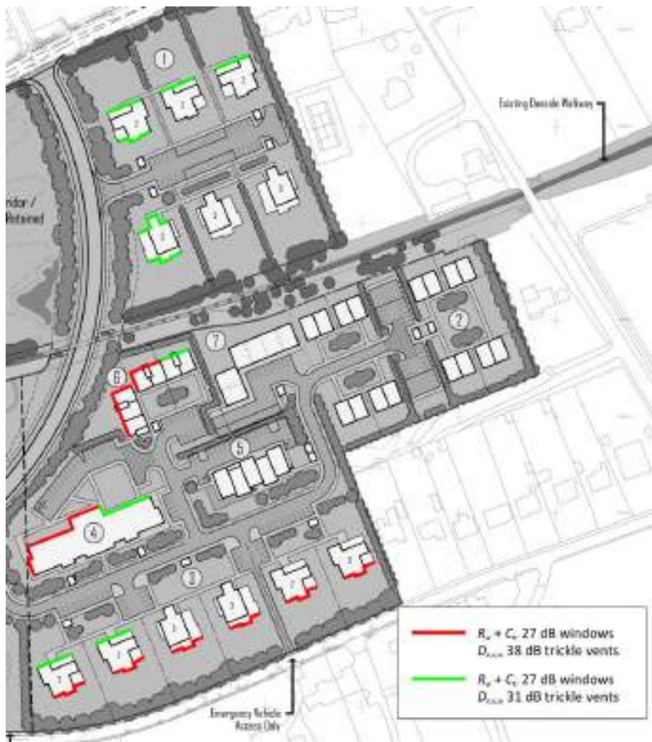
Figure 5 Facade sound insulation mark-up
