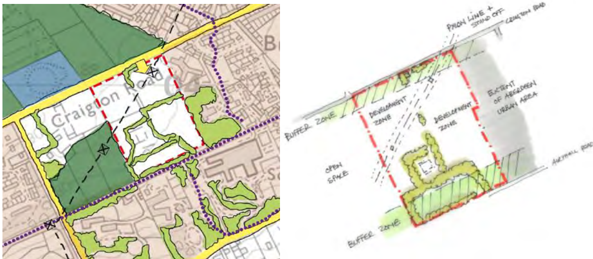
Figure 2 – Site Analysis and Design Options - retaining significant green space, woodland and site features (extracts from original Call for Sites bid document)
