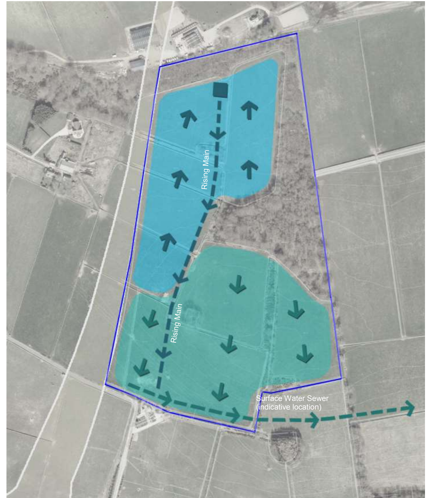
fig 67. foul drainage schematic
