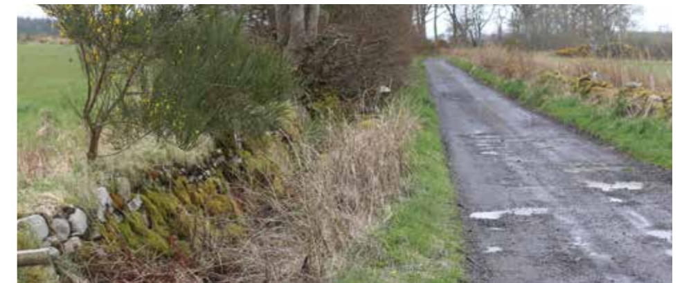
Opportunities to utilise existing walls and ditches as part of the SuDS network.
