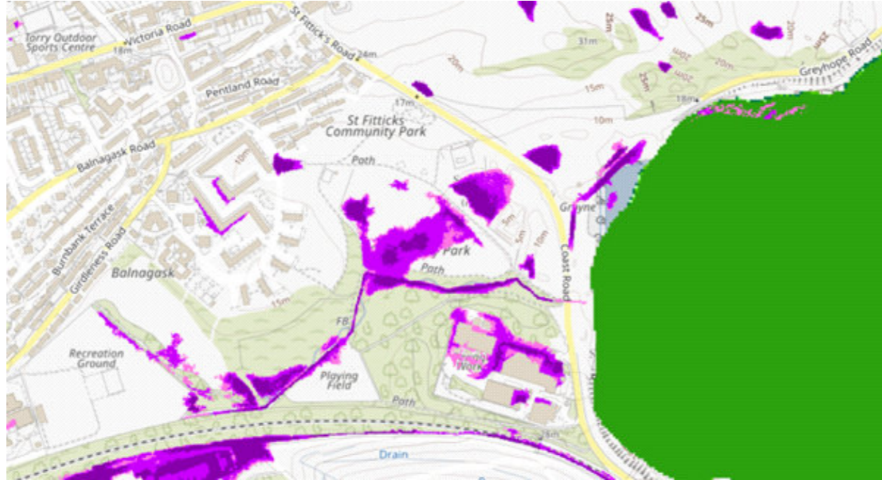
Figure 8. SEPA Flood Risk Mapping. Purple shading indicates areas currently at risk from surface water flooding. Future Flood Risk Assessment must consider potential impacts of development on local flood risk and any necessary mitigation measures.
