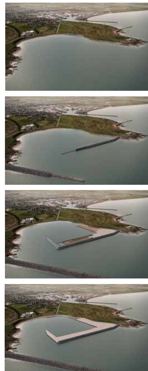
FIGURE 20 Harbour Construction Visualisations up to year 2
