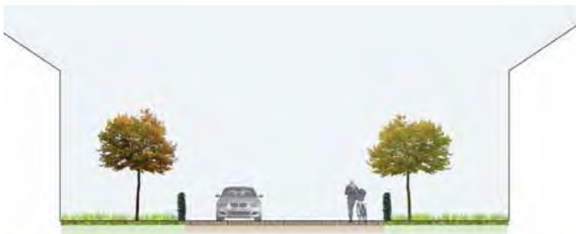
fig. 51: Indicative section: Street Type C. Shared surface.
