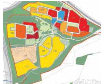
fig. 33: Scenario 3 (600 units + 100 student accommodation units) Residential higher density Residential high density Residential medium density Residential low density Residential lower density Mixed use SRUC and student accommodation
