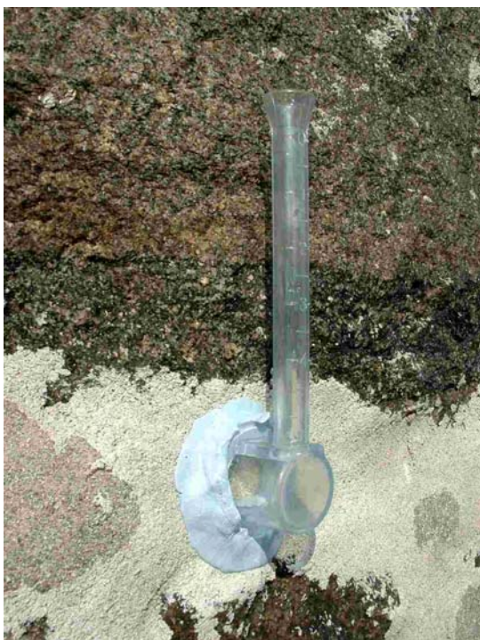
Plate 4.33 RILEM tube attached to a patch of 'lighter' mortar (Run 3).
