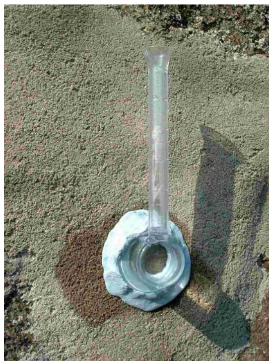
Plate 4.34 After Run 6 showing spread of water after 5mL absorption. Most water has gone deeper into the mortar; only a small proportion is visible on the surface.
