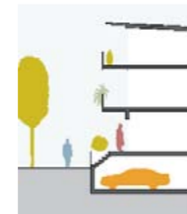
Partial underground parking with raised floor
